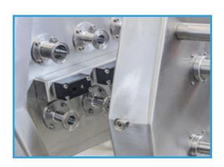
Transfer panels allow an easy and proper connection of all sanitary pipes between tanks and return line. This system allows simultaneous connections between different piping from mixers outlet. The system, composed by removable stainless steel pipes, is designed to avoid "cross contamination" in the simultaneous phases of production and CIP/SIP operation. Each pipe is equipped with inductive sensors in or-
