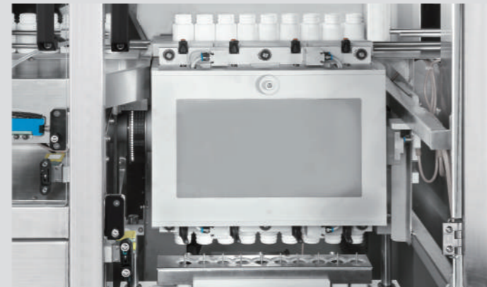
• Air Rinse Station
