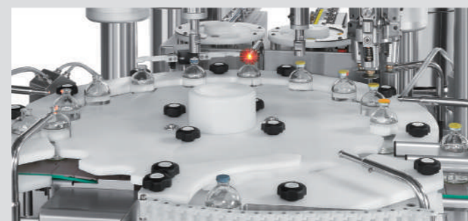
• Specialised design for eye drops provides durable compact liquid filling station, and stable operation at speeds up to 80 BPM.
