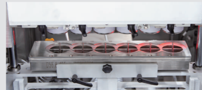
• Air Rinse Station
