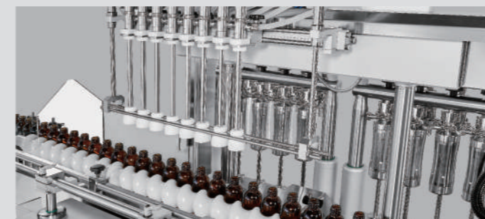
• Bottle Feed Screw System with servo motor drive.
