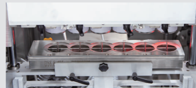
• Air Rinse Station
