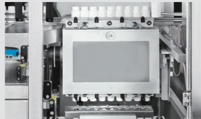
• Air Rinse Station
