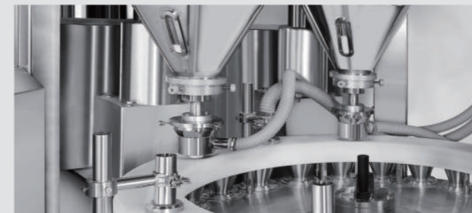
• CVC 6088-2R24: Double head auger powder filling & 24 filling station
