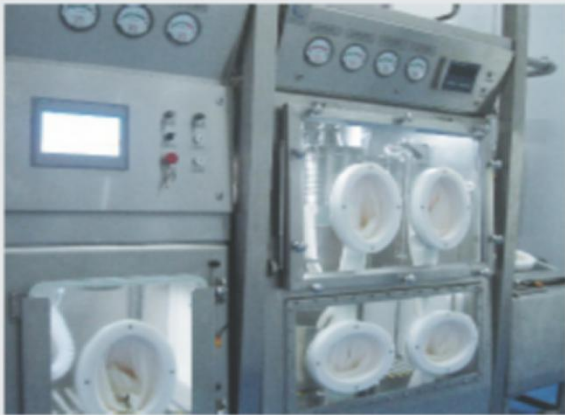
Integration isolation system with filtration, drying, weighing and filling process
