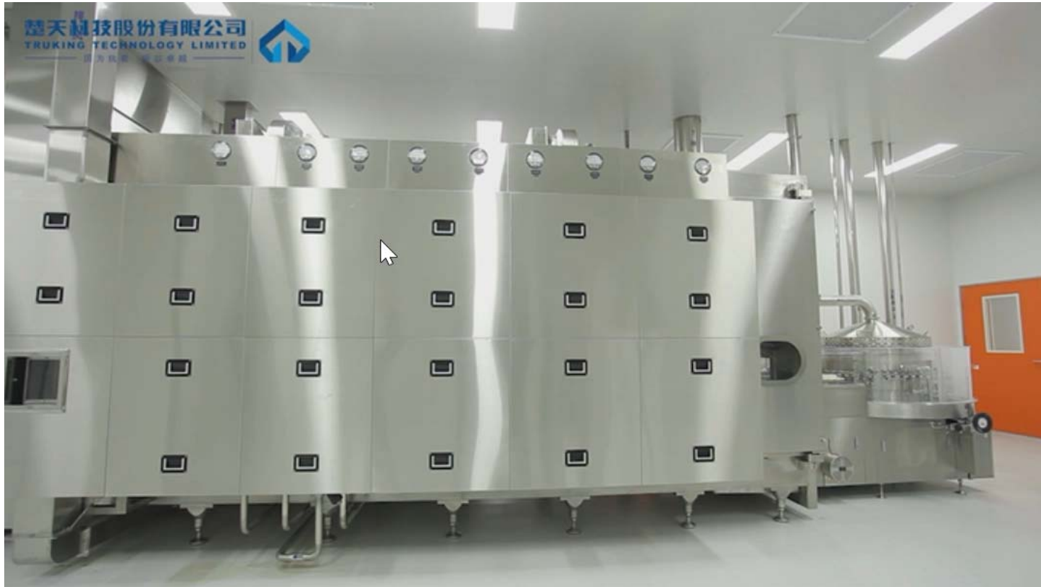
OEB5 high patent Lyophilized production overall solution with isolator
