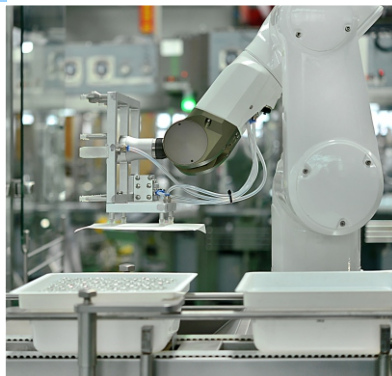
Lining paper removing
